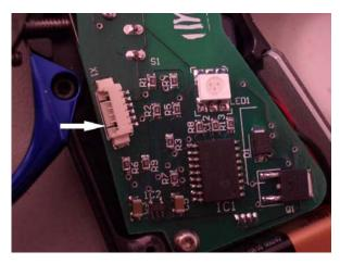
Each time the two pins are touched with a conductive object, such as a hex wrench, the LED will briefly flash green or red to indicate the status of the programming mode. If it flashes green, programming mode is allowed. By default the tournament lock is disabled, allowing the user to change settings.
