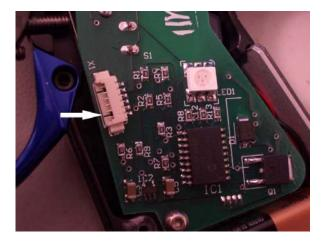
Each time the two pins are touched with a conductive object, such as a hex wrench, the LED will briefly flash green or red to indicate the status of the programming mode. If it flashes green, programming mode is allowed. By default the tournament lock is disabled, allowing the user to change settings.
