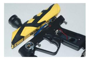
Remove the front pneumatic fitting with a 1/8" Allen wrench. Make sure to remove the pneumatic fitting from the hose afterwards and set it aside.
