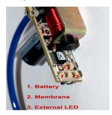
As shown in the above diagram, there is a specific socket for a membrane pad harness and external LED harness. Both harnesses can be purchased separately, if needed, and allow for easy installation of the desired accessories.
