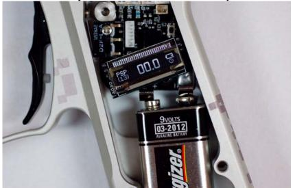
Completed installation of board and battery:
